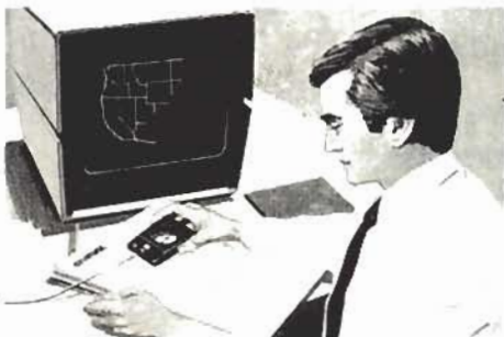
Figure 4: A typical graphics tablet or digitiser. The pen can be used to trace an outline and send the co-ordinates of points back to the computer.
